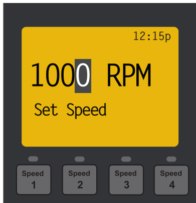
Setting the Anti Freeze Pump Speed
