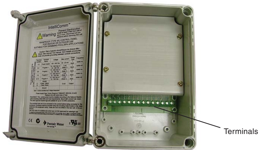
IntelliComm Communication Center
